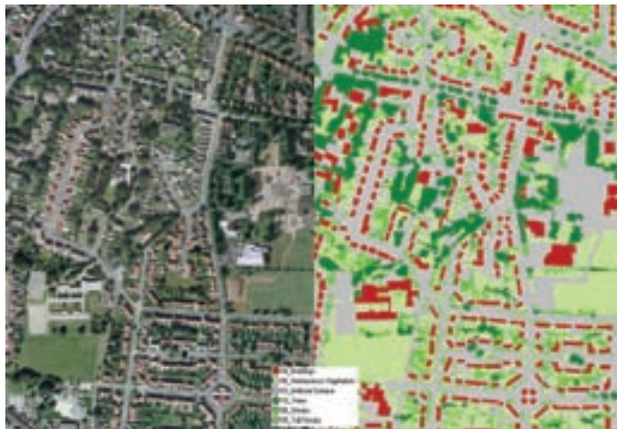
LandBase Level 2 classification over Derby City Centre, utilising lidar height information to further improve classification accuracy.
