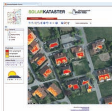
Fig.4: WebGIS screenshot of an SUN-AREA online solar potential map of Worms (Germany)
