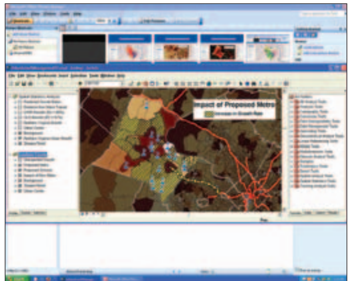
FIGURE 3. ArcGIS Spatial Analyst helps the researcher see how a proposed metro extension will affect urban growth. This aids planning decisions such as highlighting where new schools will be needed.
