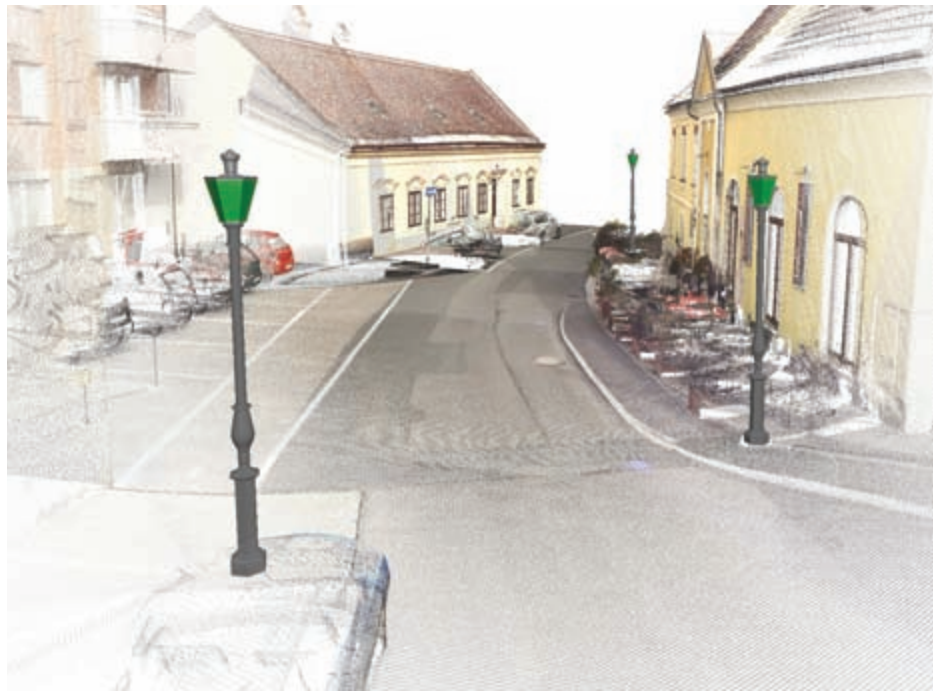
Fig.4: The clean-up of point cloud data using Bentley Descartes' classification editing enables the creation of a hybrid information model (data acquired with RIEGL VMX-250 Mobile Laser Scanning System)
