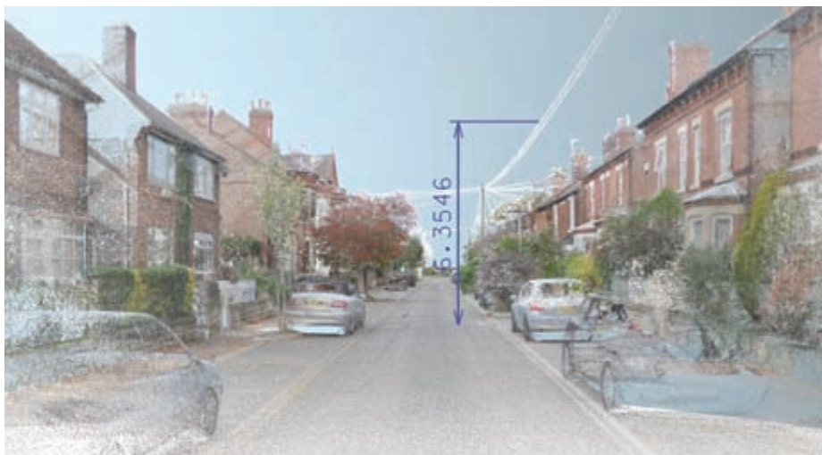
Fig.5: Point clouds enable 3D visualisation as well as the measurement of assets (data captured by StreetMapper)
