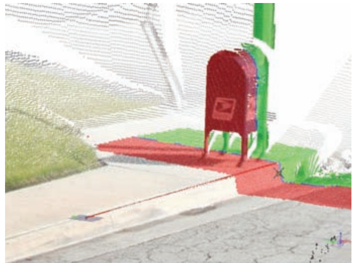
Fig.3: Dynamic sectioning in Bentley Descartes for land surveying (data source www.libe57.org © 2010, McNeil Engineering)
