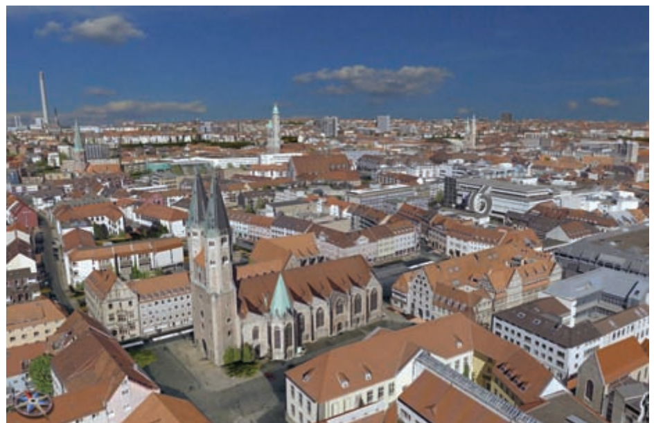
Fig.2: Texturised 3D city model of Braunschweig in Lower Saxony, automatically generated from stereo aerial photographs captured by IGI's Quattro DigiCam Oblique camera. Courtesy of 3D RealityMaps/AeroWest
