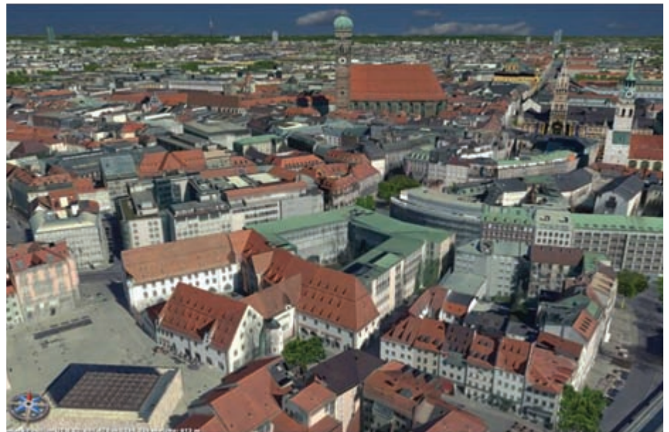
Fig.1: Photo-realistic 3D-city model of Munich automatically generated from stereo aerial imagery.
