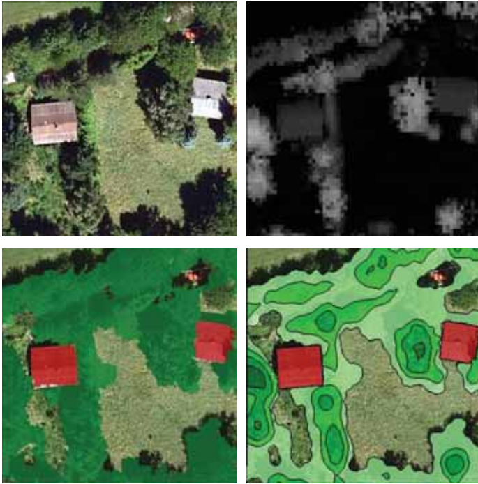
Figure 5. upper left: RGB; upper right: nDSM; lower left: basic land cover; lower right: generalized results
