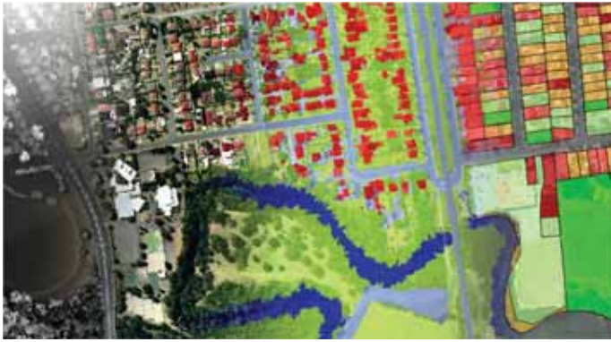
Figure 1. Airborne photography, LiDAR data and GIS vector information is fused to generate impervious surface maps on a cadastral level]
