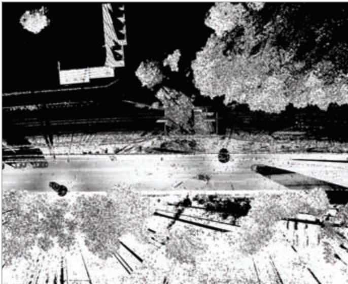
Vertical scan of accident scene The positioning and visibility of road signage is often an important factor in accident investigations
