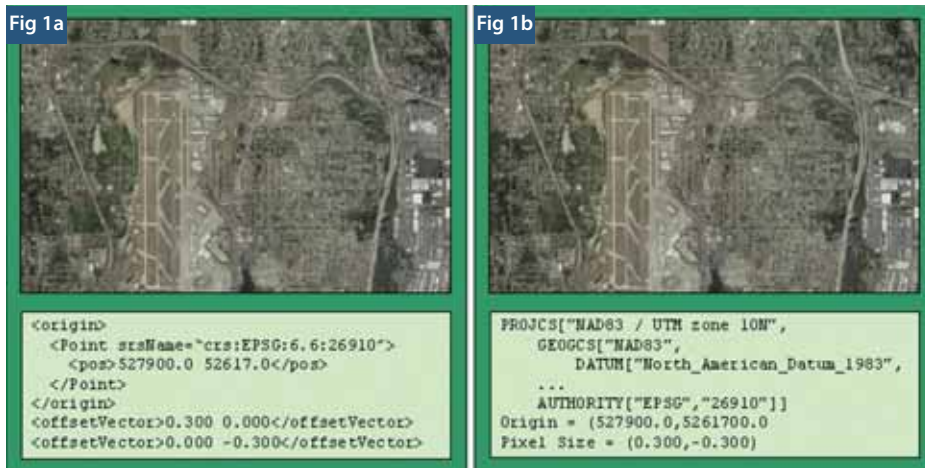
Fig. 1a - a JP2 file containing image data and GML georeferencing data Fig. 1b - a GeoTIFF file, with the same information.
