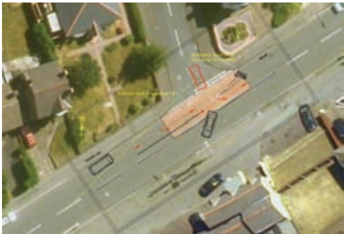
It is straightforward to overlay the information from a Police scene survey plan onto an aerial image for analysis of the accident. NOTE that the accident shown here is an imaginary example for illustration purposes and does not show an actual incident" © Copyrite Blom Pictometry 2006
