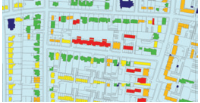
Fig 1 - Thermal aerial mapping - different colours for relative heat loss from buildings. Red and orange are high, yellow is average and green and blue is low.
